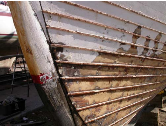
Splines in place ready to be planed and sanded
