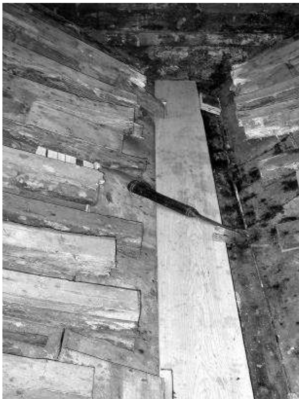
Fig. 2 The ribs were cut back and the top 50 mm of keel was chiselled away. A new top to the keel, made from three laminated layers of hardwood, was screwed down and sealed to be watertight. When the top of the keel was exposed, a slit for a centreboard was discovered.
