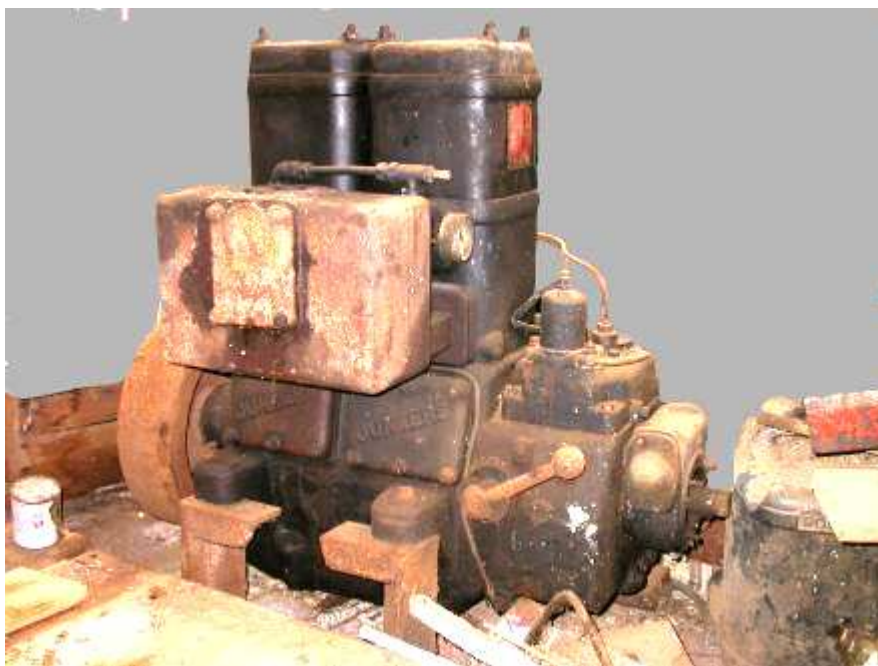
Bob Jager's HK65 Junkers engine. There are two cylinders vertically arranged, with two pistons in each cylinder.
