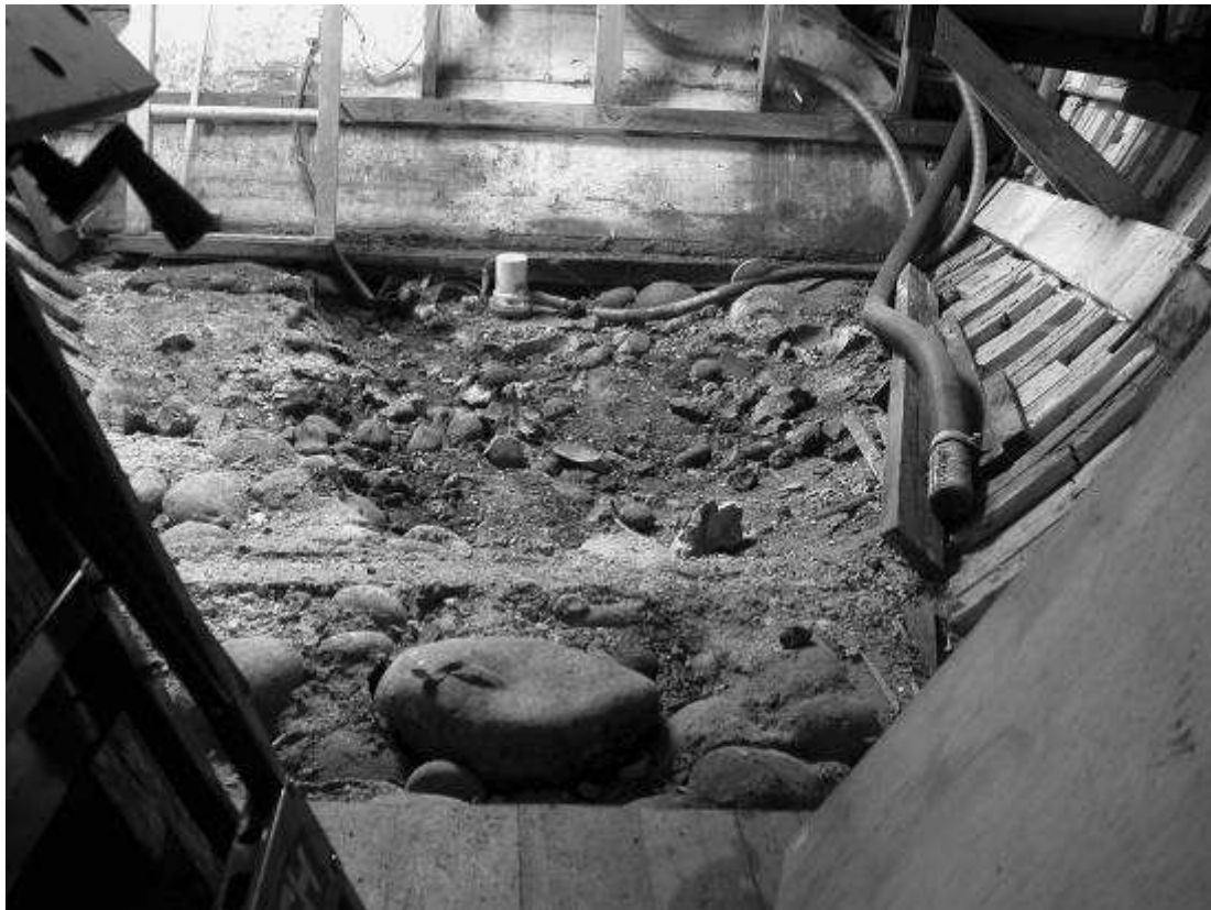
Under the sole in the fo'c'stle was revealed ballast of river boulders, rusty iron and crumbly concrete
